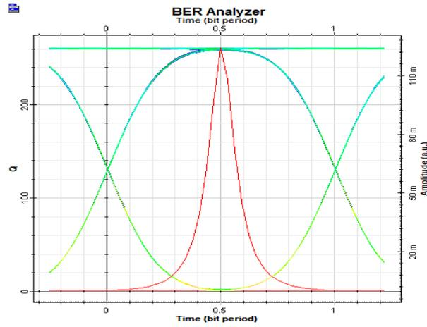
Fig 3:Eye pattern for NRZ at 1550nm for 5Km transmission.
