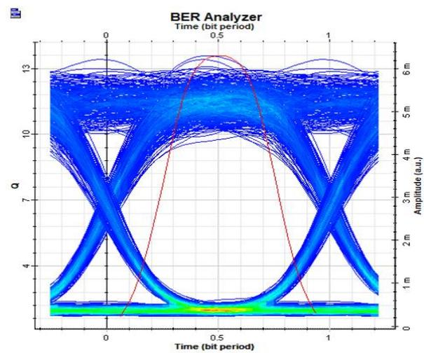
Fig 5: Eye Pattern for NRZ at 1550 for 50 Km transmission
