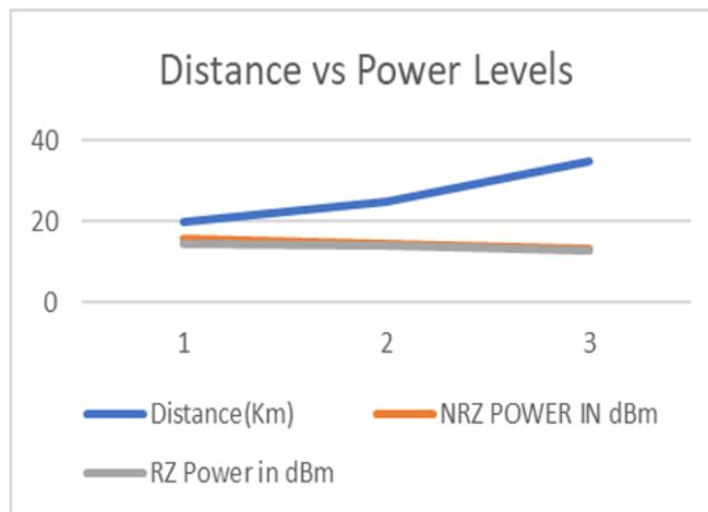
Fig 13: Distance vs Power levels for RZ &NRZ
