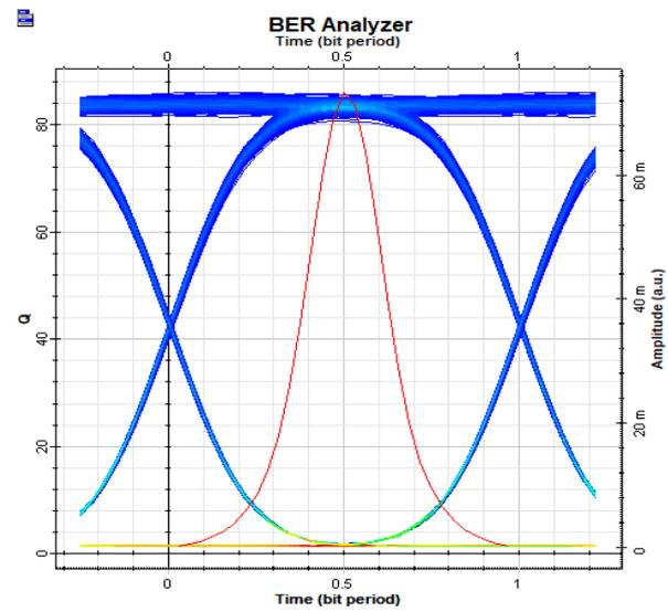
Fig 4:Eye Pattern for NRZ at 1550 for 20 Km transmission
