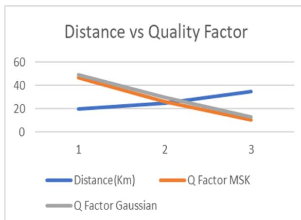
Fig 14: Distance vs Quality Factor for MSK & Gaussian modulation Formats.
