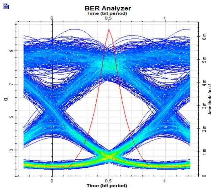
Fig 11: Eye Pattern for MSK at 50 Km
