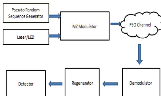
Fig 1: Block Diagram Representing the FSO System
