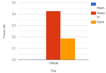
Fig 5: Power occupied by different operating modes in 1 minute
