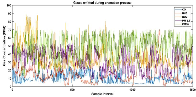
Fig 8: Concentration of different gases emitted during cremation process
