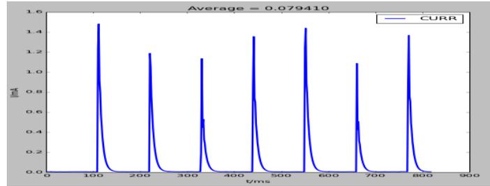
Fig 11: Average power consumed by ESP 32 when acquiring data periodically ( 30samples per minute)
