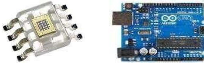
TCS8200 (R.G.B SENSOR) (Fig-1) ARDUINO UNO (Fig2)
