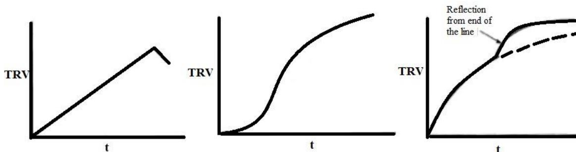
Figure 2.2 (a) Triangular TRV (b) I-Cosine TRV (c) Exponential TRV
