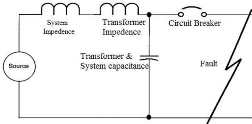
Figure 2.1. Simplified TRV circuit representation
